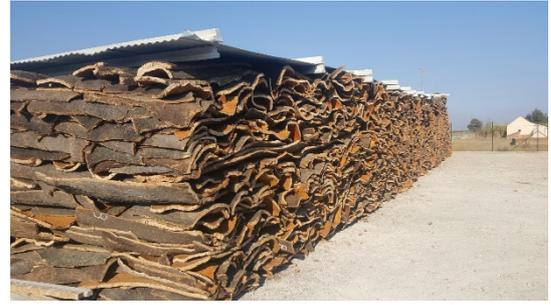
Once the cork has been adequately seasoned, the bark is brought to the factory for boiling. Boiling helps to flatten the cork planks, eliminate insects, and sterilize the cork. The process also helps to expand the cork wood cells, which increases the thickness and smoothness.
