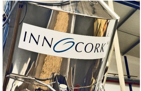
Innocork uses ethyl alcohol, which is a safe, natural agent that is common to wine. Using controlled conditions to maximize extraction and prevent re-absorption allows Innocork to mimic the natural organic chemistry that can occur inside of a wine bottle if releasable TCA were present in the bottle's cork.
